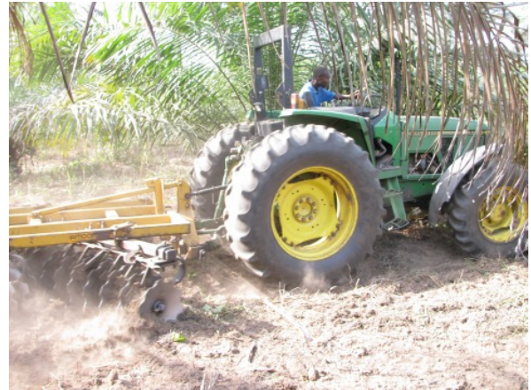
Figure 6: The John Deere 6400 tractor and heavy duty harrow in operation on Omodeni Farm.
