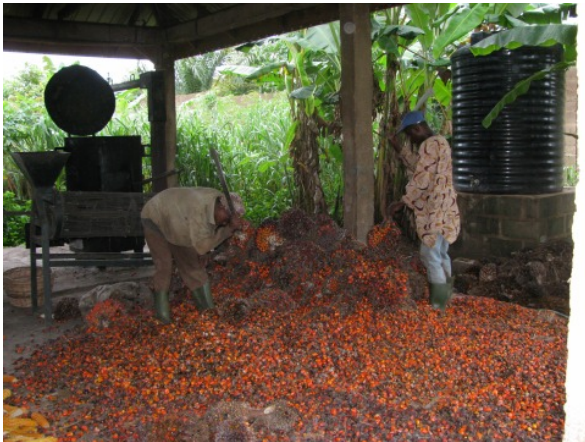
Figure 9: Paul and Tope splitting fruit. After splitting, the fruit is sent through the cleaner and then into the sterilizer.
